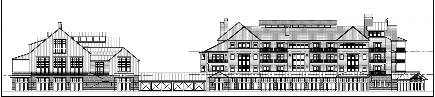
NEW SKIER SERVICE BUILDING NORTH/SOUTH ELEVATIONS
